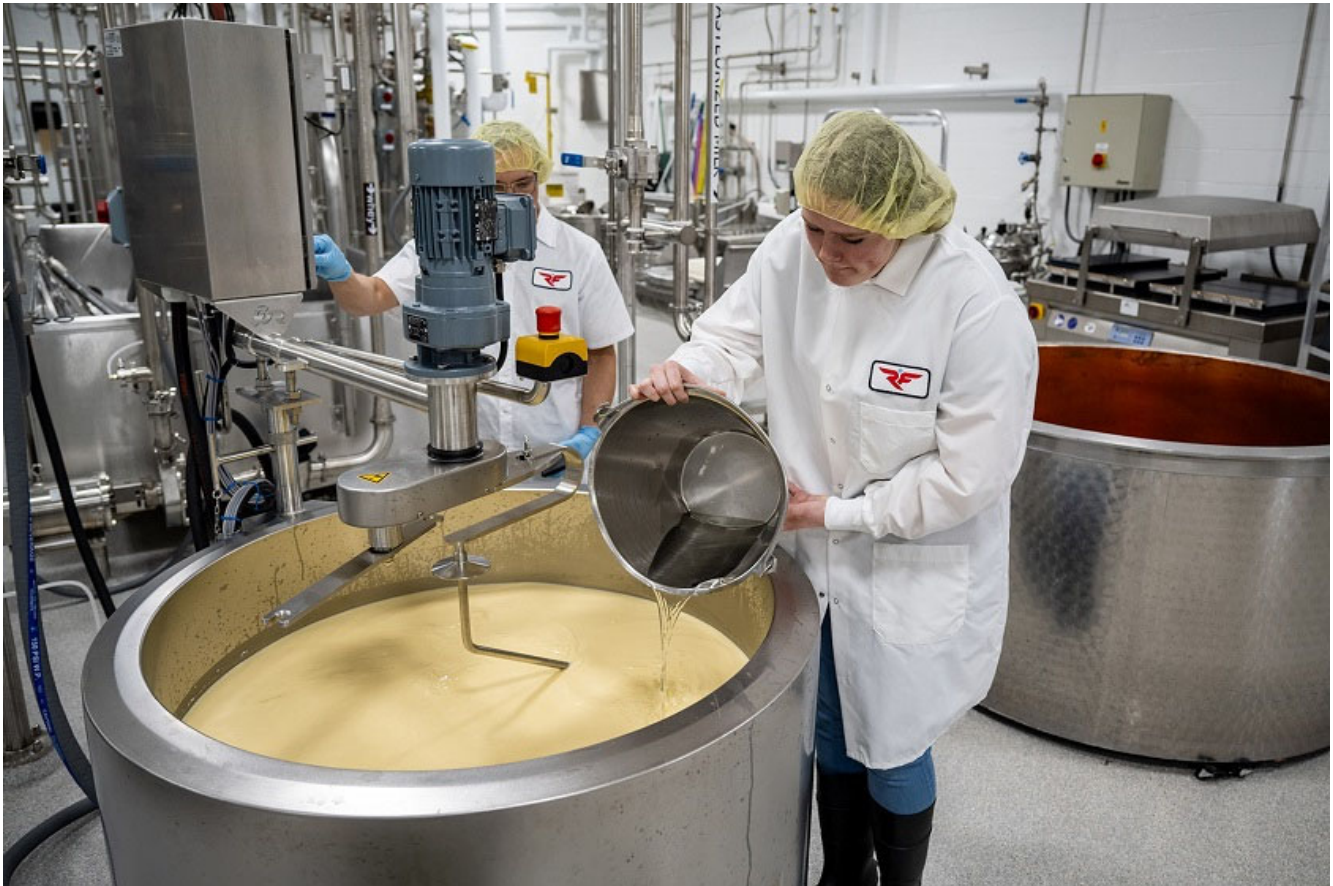
UW-River Falls junior Makenzie Skibbie adds rennet to a batch of cheddar cheese being produced Tuesday at the university’s Wuethrich Family/Grassland Dairy Center of Excellence. Rennet promotes curdling, helping transform milk into cheese. UWRF/Pat Deninger photo.
