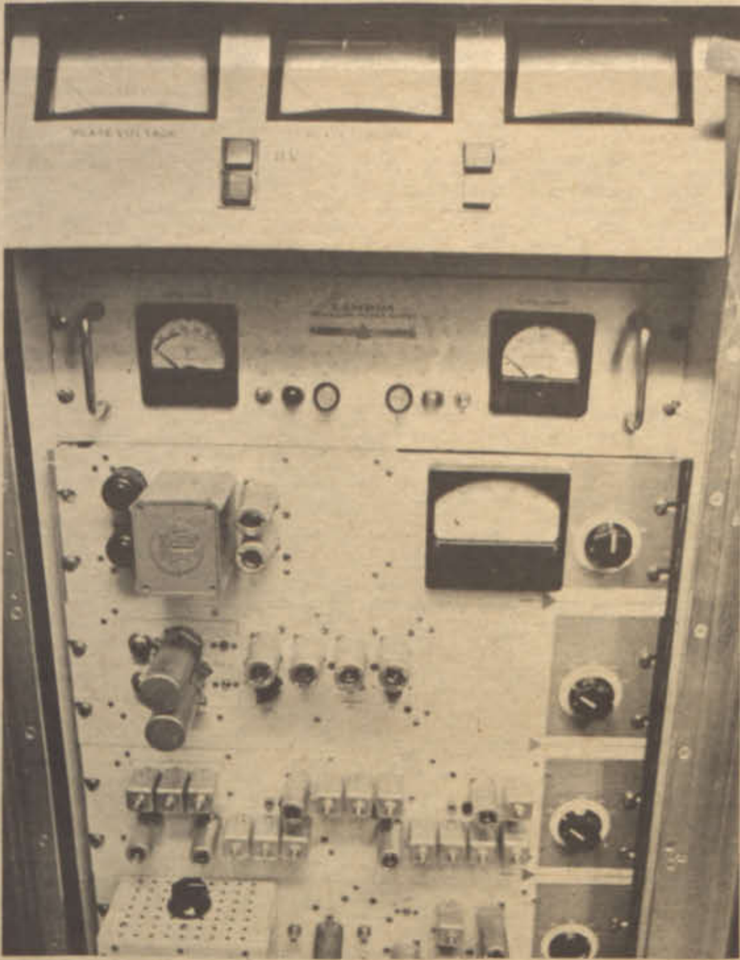
WRFW's new 1000-watt transmitter awaits installation at the station's new tower site soon to be under construction. Photo by Mike Ray.
